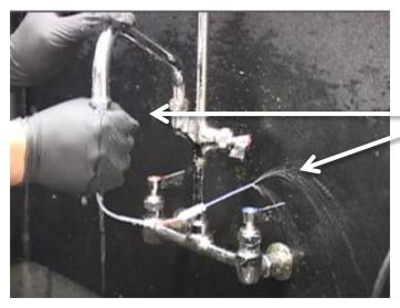
This picture clearly shows that the injectors are not clogged. To achieve this you may need to wear gloves to create a seal. The water faucet should be on a little above a trickle.
